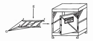
5. Insert the shelf (E) and bolt it to the shelf support rail using bolts, washers, and nuts provided (G & H).
