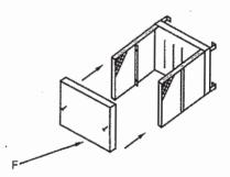
2. Assemble the top panel (F) to the side panels (D). Hand-tighten the bolts, washers, and nuts provided (G & H). Ensure the unit is square and firmly tighten the bolts connecting the side panels to the base. Tighten the bolts connecting the side panels to the top panel. Set unit upright.
