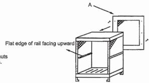
3. Connect the back panel (A) to side panels (D) using bolts, washers, and nuts provided (G & H). Ensure the unit remains square and firmly tighten the nuts. Note: out of square assembly will prevent the door from closing properly.
