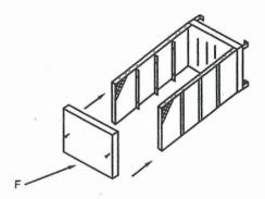
2. Assemble the top panel (F) to the side panels (D). Hand-tighten the bolts, washers, and nuts provided (G & H). Ensure the unit is square and firmly tighten the bolts connecting the side panels to the base. Tighten the bolts connecting the side panels to the top panel. Set unit upright.
