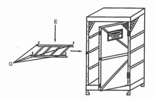
5. Insert the shelves (E) and bolt them to the shelf support rail using bolts, washers and nuts provided (G & H).
