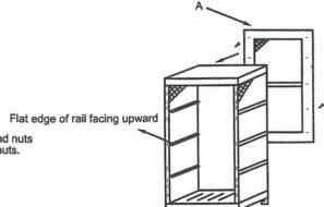
3. Connect the back panel (A) to side panels (D) using bolts, washers, and nuts provided (G & H). Ensure the unit remains square and firmly tighten the nuts. Note: out of square assembly will prevent the door from closing properly.
