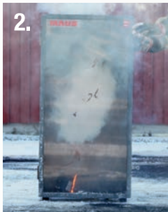
2. Once the battery was on fire it activated the HDC cable that activated the MAUS unit in the ceiling.
