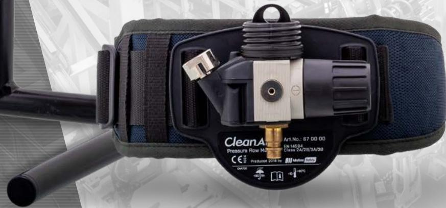
Systems CleanAIR® Pressure/Pressure Flow Master are constant flow supplied air respirators suitable for a long term work in the heaviest industrial environments. The regulator on the belt unit can adjust the amount of air coming from the central compressed air distribution system or a compressor and keeps it at a constant level without regard to the changes of inlet pressure.
