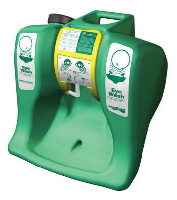
**Application:** Self-contained 16 gallon gravity-flow eyewash unit is ideal for use in low traffic areas, and where a continuous supply of potable water is unavailable for plumbed units. Rugged plastic tank is wall mountable near any hazard. Unit uses gravity to deliver approximately eight gallons (30 liters) of water for 15 minutes through dual spray heads, thus complying with the provisions of ANSI Z358.1-2014 for eyewashes.
