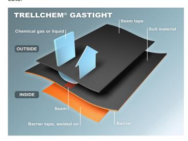
In a traditional seam, made on a material with the *Barrier film embedded* inside the material, it becomes *impossible to seal* it, thereby creating a weak spot in the seams where the chemicals can permeate. This explains the often shorter seam permeation times shown for these type of seams, compared with the suit material itself! See the scetch below.
