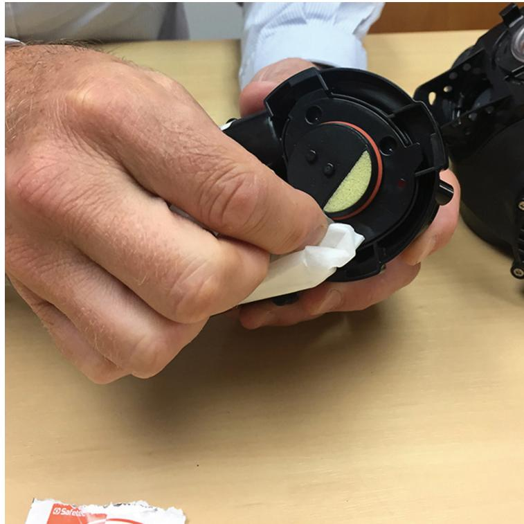
Check the Inhalation valve on the back of Fan Unit ensuring there are not tears or signs of damage. This part can be replaced if required (see Instruction Manual for part numbers). Check Guarding Sponge is intact. This part can be replaced if required (see Instruction Manual for part numbers).
