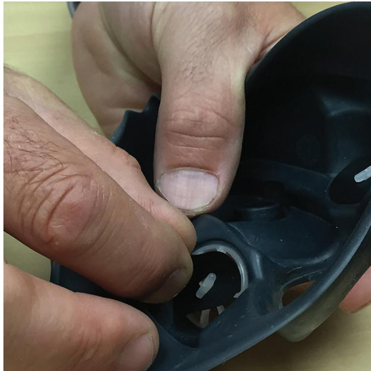
Check Drain Valve and replace if necessary.
