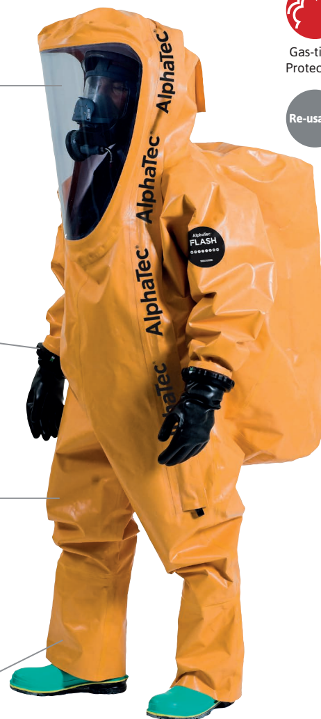
Strong and flexible suit material with excellent abrasion and flame resistance, provided by the aramid base fabric and the outer layer of chloroprene rubber
