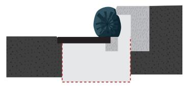
Ensure that all gaps and holes are blocked between the kerb channel and catchpit protection.
