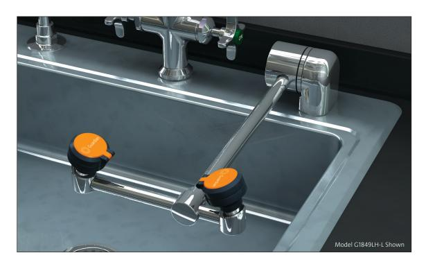
**Application:** AutoFlow<sup>™</sup> eyewash for mounting on counter. Spray heads swing down from storage to operational position, activating water flow. Available in a variety of spray head configurations to minimize obstructions at a sink. *Note: If unit is not installed at a sink, floor drain should be provided underneath unit to prevent accumulation of water on floor.*
