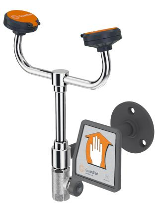
Application: Eye/face wash for wall mounting. Two large FS-Plus<sup>™</sup> spray-type outlet heads deliver a flood of water for rinsing eyes and face. Unit is provided without bowl or drain for waste water. Note: Floor drain should be provided underneath unit to prevent accumulation of water on floor.
